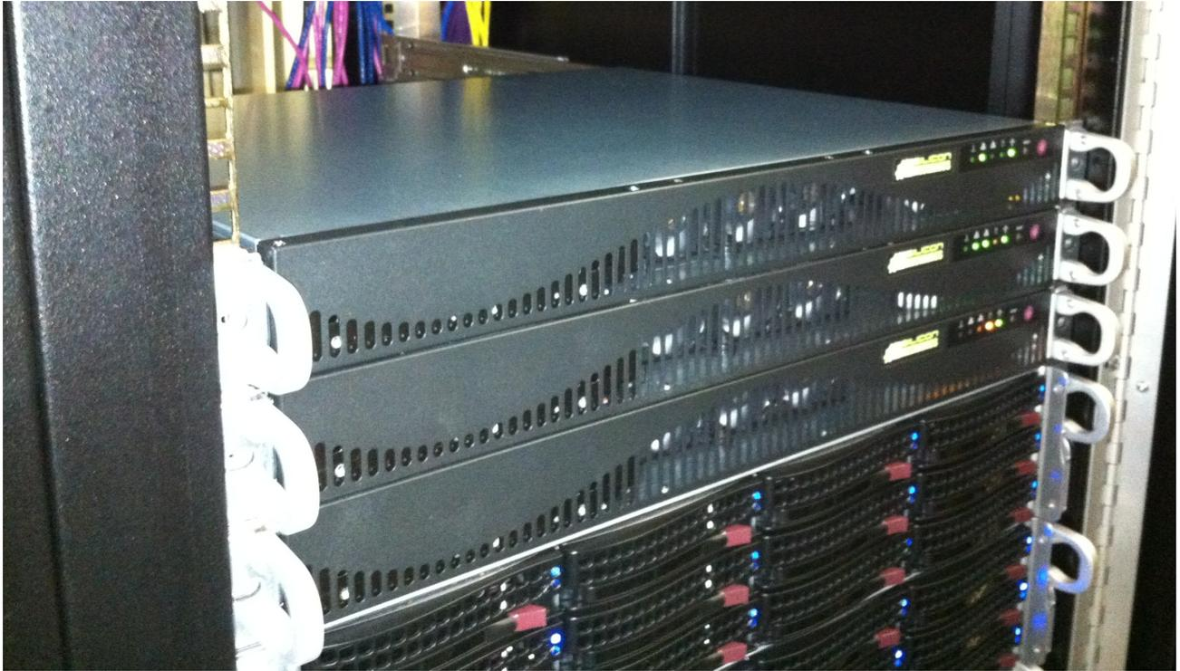
The trio of new servers configured for the high-availability Linux Virtual Server (LVS) environment and LDM Ingest Data at Penn State.
